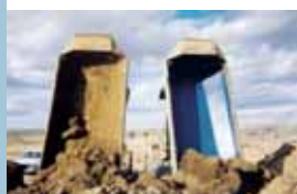
Better release No friction: Truck lining of OK 2000 blue 588.
