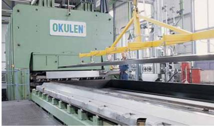
Using our state of the art CAD technology we support our customers engineering requirements in the development of complex components. In self designed twin-levelpresses we produce semi finished components in thicknesses from 6 to 400 mm (1/4 to 15 3/4 inches).
